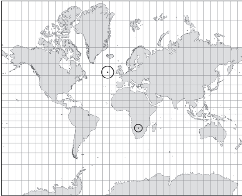
FIGURE 5.11. Two Tissot indicatrix circles shown on a Mercator projection with the standard line of the equator.
