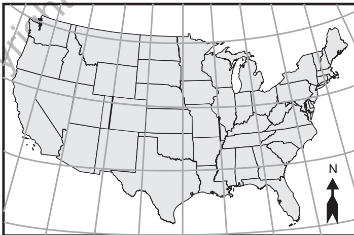
FIGURE 2.21. North arrows should not be used if meridians radiate or curve. The arrow on this conic projection does not point north.
